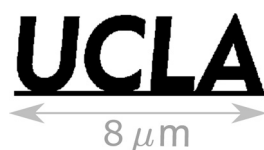
FIG. 4. The geometry of the target used for mass contrast imaging is shown in black, and a scale bar is shown in gray. In order to calculate the effect on the electron beam (angle scattering and energy loss), the sample is assumed to be a 20\text{ }\mu\text{m} thick Cu.
