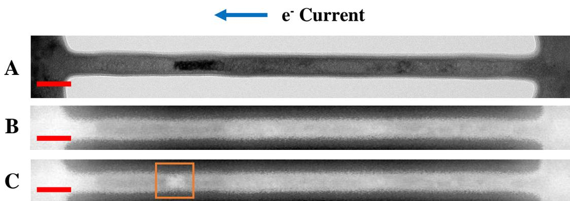
**Figure 2.** **A)** BF STEM image of an Al/Cu nanowire before biasing. The macro-scale defect where copper later accumulates is clearly visible. **B)** DF STEM image of the same nanowire before biasing. **C)** DF STEM image of the nanowire after biasing. A mass appeared near the macro-scale defect (indicated by an orange rectangle), and is identified as copper by EDS analysis. Scale bars are 50 nm.
