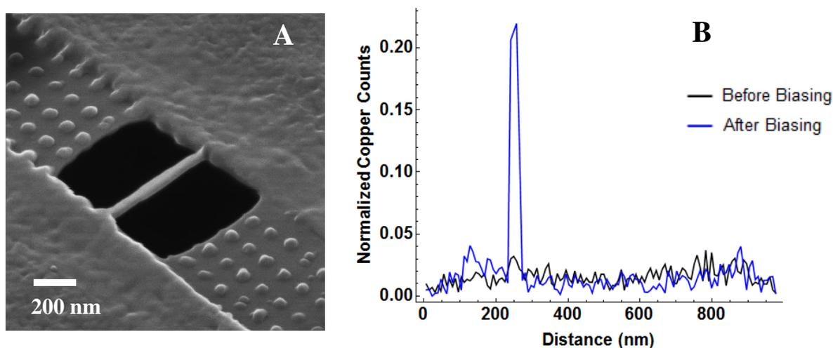
**Figure 1.** **A)** Tilted-SEM image of a helium-ion milled wire. The nitride support film and some alloy islands surrounding the Cu/Al alloy wire have been removed by milling. **B)** EDS copper profiles along the wire axis before and after biasing. A large spike in copper counts appears after biasing. Copper counts are normalized to aluminum counts since the aluminum count rate was unchanged.
