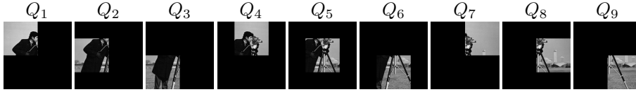
FIGURE 4. Scanning positions generated by the illumination windows described in Section 4.1.2. For the small problem where n_1 = n_2 = 512 (Section 4.1.1), each illumination window Q_i has size 256 \times 256 and shifts 128 pixels at a time. Similarly, for the large-scale problem where n_1 = n_2 = 16384 (Section 4.1.4, each illumination window Q_i has size 8192 \times 8192 and shifts 4096 pixels at a time. In both setups, there is a 50% overlap between consecutive probes.
