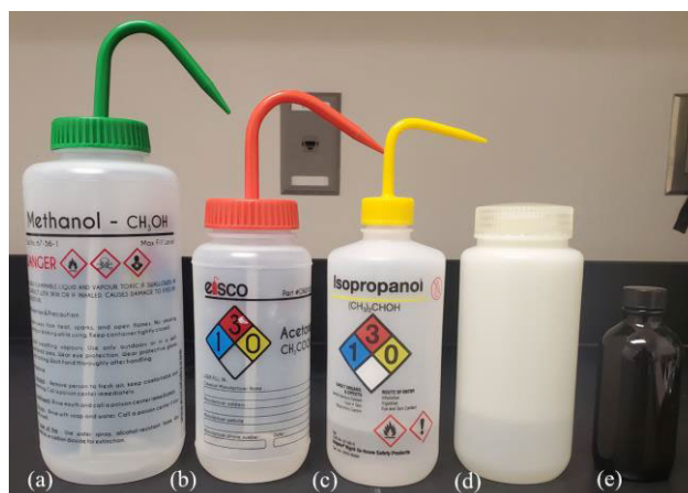
Fig. 1. Common storage containers: (a)–(c) LDPE squeeze bottles, (d) HDPE jar, and (e) amber glass jar.
