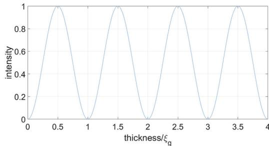
Figure 2: Plot of intensity variation in primary beam as thickness varies from 0 to 4 extinction lengths  $\xi_g$ .
