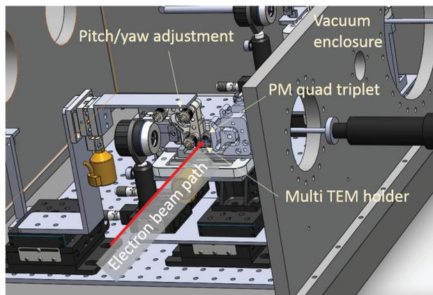
Figure 5: Experimental setup at UCLA showing UHV chamber containing TEM holder in which grating will be mounted, permanent magnet quadrupole triplet to image the diffracted beam, and related equipment.
