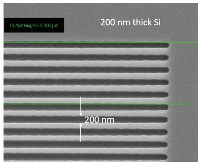
Figure 4: Example Si grating with 400 nm period and 200 nm thickness, courtesy of Norcada.
