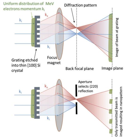
Figure 1: Upper diagram shows electron beam diffracting through crystal in two-beam condition and forming image downstream. Lower diagram shows how image changes if one of the diffraction spots is blocked. The image is then only of the grooves or ridges in the crystal, producing a nanopattern in transverse density, which may be magnified or demagnified with conventional optics.
