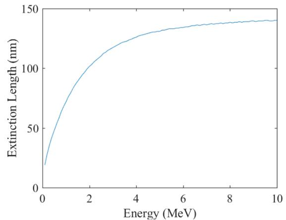
Figure 3: Extinction length vs beam energy including relativistic effects. The extinction length depends on velocity rather than energy.
