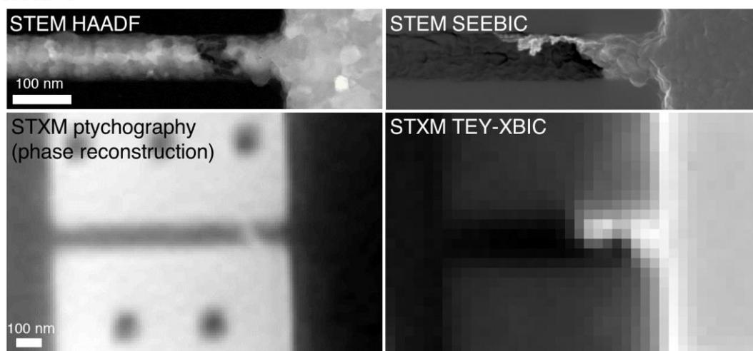
**Figure 1.** STEM HAADF and SEEBIC images and STXM ptychography and TEY-XBIC images of a damaged Al wire. The (upper) STEM images were acquired with 80 kV electrons and the (lower) X-ray images were acquired with 1565 eV photons. In each beam-induced current image, current is measured from the right Al electrode and the left electrode is held at ground. Bright/dark contrast in the induced current images corresponds to positive/negative (hole/electron) current.
